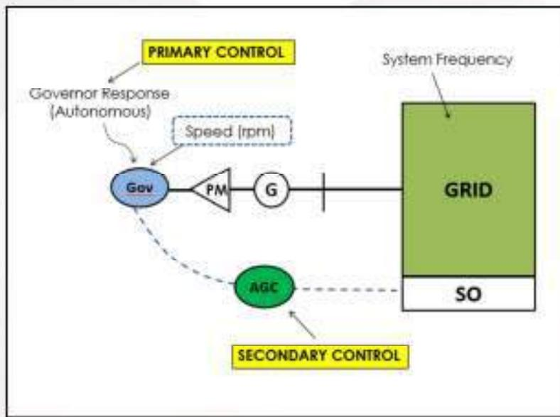
*Figure 2 - Difference of Primary Control and Secondary Control*
