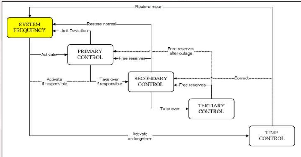
*Scheme and actions starting with the system frequency*
